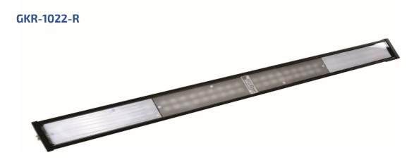
The <u>GKR-1022-R (LED Light Rail)</u> (page 19) works in conjunction with the GKR-1020 to capture the undercarriage imagery. Each GKR-2011 IVUS System contains two (2) LED Light Rails. When triggered, each GKR-1022-R floods the underside of the vehicle with a distinctive red light. This component is installed on both sides of the GKR-1020 inside the GKR-1043-2.
