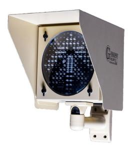
The <u>GKR-7080 (Traffic Control Signal Light)</u> (page 20) controls vehicle traffic crossing over the GKR-1020. Once triggered, the GKR-7080 will change from a green arrow to a red X. This controlled entry into the GKR-2011 IVUS System helps to create accurate imagery of the under carriage and over view. The GKR-7080 is placed on the GKR-1086.
